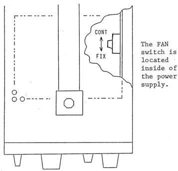
Turn off the POWER switch and throw the FAN switch to the FIX position using an insulative small rod. The FAN will start unconditionally as the POWER switch is turned on.
