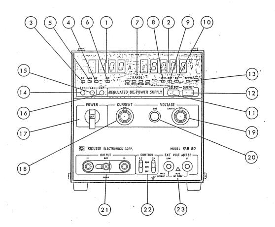
(13) OUTPUT lamp: Indicates that the output is in the ON state.
